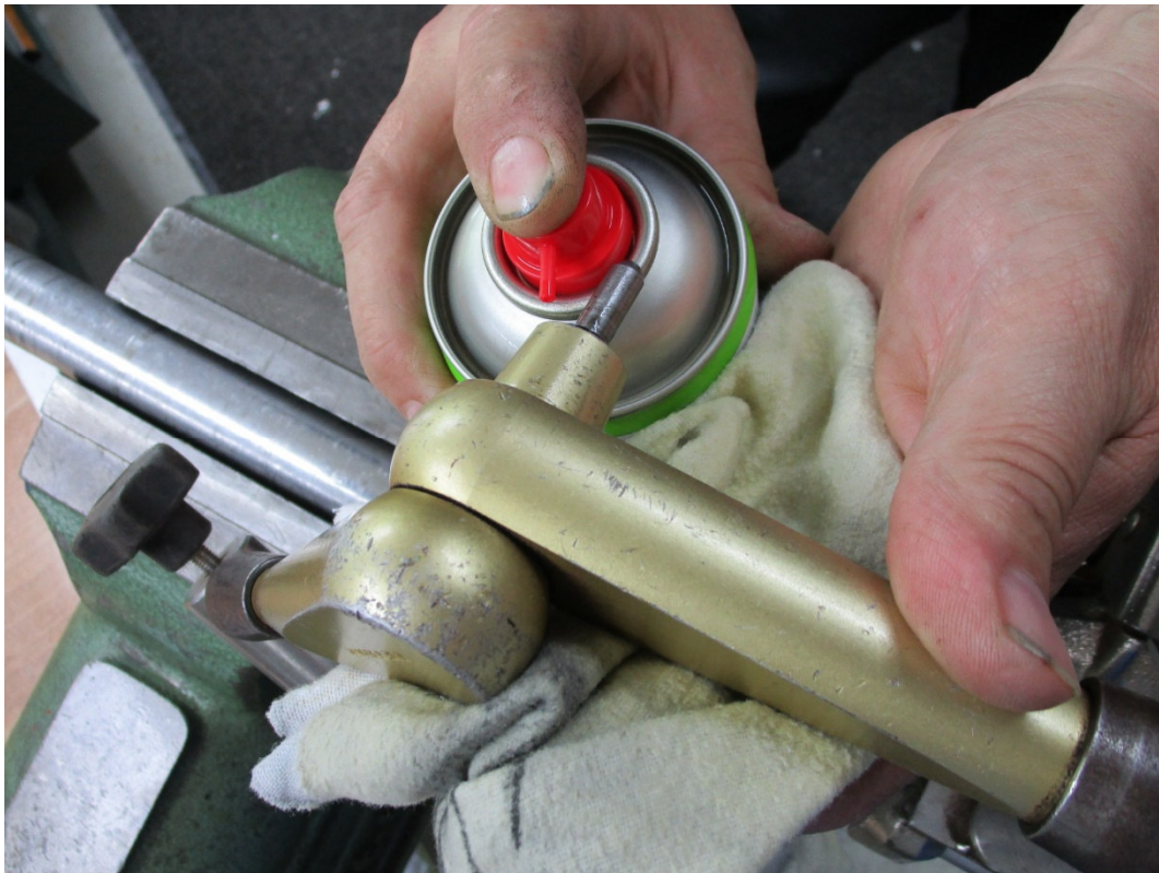
10) Clean and degrease the joint.
