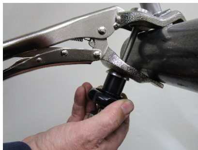
turn the clamping cone tightly with the black handwheel
