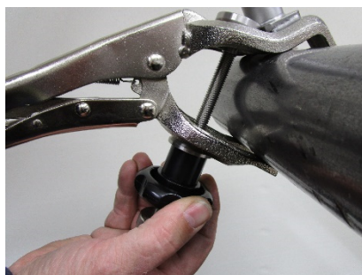
to release the locking spindle again, the pliers should be clamped
