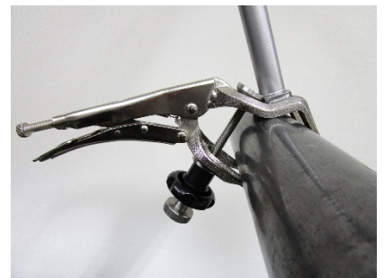
until the jaws are jammed - now the gripper is secured against rotation
