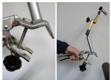
when the handwheel is loosened, the gripper can be opened
